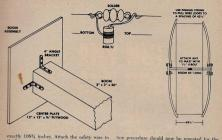
the loop at each pole and solder. The side with the insulator is measured and assembled last. This side of 108% inches will include the length of the insulator. Since the safety wires have been soldered on the ends of this side, adjust the length by pulling the ends of the wire through the insulator and wrap the wires tight. Do not solder
